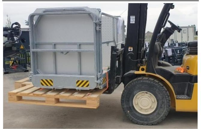
The full package can be lifted either by lifting the pallet on which the platform is fixed as shown, or by lifting only the platform by the two slots (pockets) under its floor.
