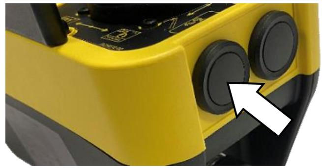
In the event the operator at height is unable to carry out these instructions, a second operator can intervene from the cab by pressing the red emergency pump activation button with dedicated graphics, which is located on the dashboard to the right of the driver's seat.
