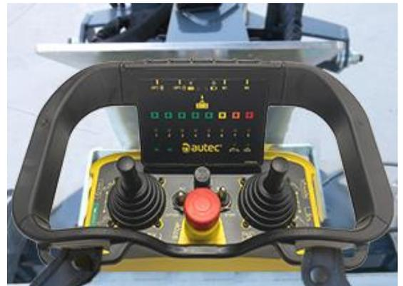
All movements made by the vehicle driver from the driver's cab are limited in height and boom extension movements so that the equipment can be coupled to/uncoupled from the boom of the vehicle when it is on racks or loading beds of transport vehicles.
