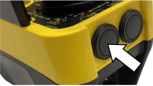
In the event the operator at height is unable to carry out these instructions, a second operator can intervene from the cab by pressing the red emergency pump activation button with dedicated graphics, which is located on the dashboard to the right of the driver's seat.
