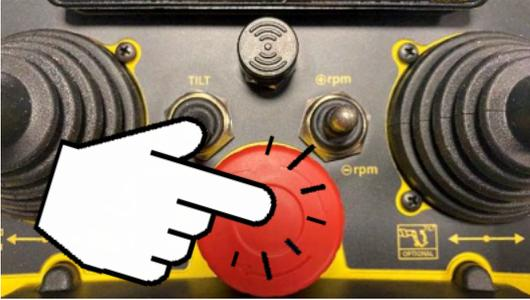
To re-enable the platform controls, switch on the radio control by turning the red emergency button clockwise and repeat the connection procedures given above.
