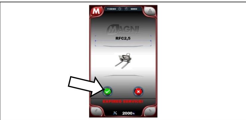
**If the accessory is not recognised, check the state of preservation of the signal transmitter present on the accessory and of the signal receiver present at the head of the boom. If there is no damage, contact the Magni Telescopic Handlers Assistance Service.**
