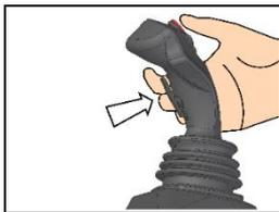
Inside the grip of each servo control there is a button with the “**movement enable**” function: press this button to impart a command to the forklift truck or accessory attached. Absence of the procedure is displayed on the control panel
