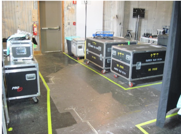
Fig. 4-1 – Marked fire aisle to door. When loading, moving and storing equipment and equipment containers, it is easy to forget that an aisle must remain open for egress. Marking the aisle with bright tape helps remind everyone that an aisle must be maintained to allow for access to the exit. Keeping the marked area completely clear is an important part of an effective safety culture. Photo courtesy of Steve Lemon.
